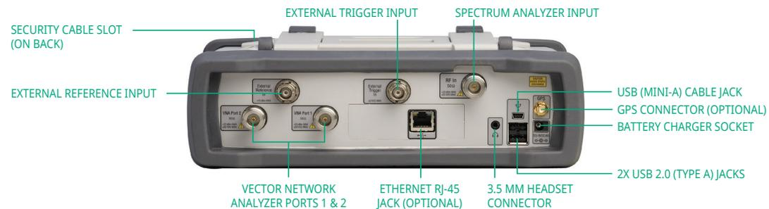
ALL CONNECTORS ARE CONVENIENTLY LOCATED ON THE TOP PANEL, LEAVING THE SIDES CLEAR FOR HANDHELD USE
